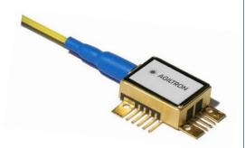
The FORX Linear Photoreceiver is designed for high-speed and high sensitivity analog and digital applications, featuring a surface-coupled coplanar waveguide APD photodiode and a linear transimpedance amplifier within a hermetically sealed package. Its high conversion gain and low input-referred noise ensure exceptional linearity and precision.
